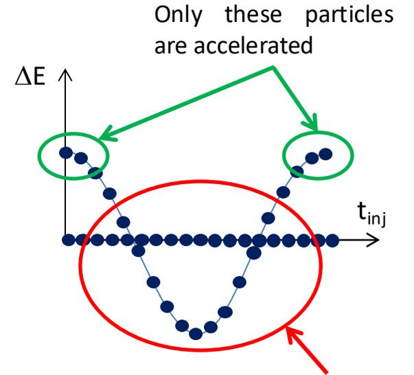
These particles are not accelerated and basically are lost during the acceleration process
