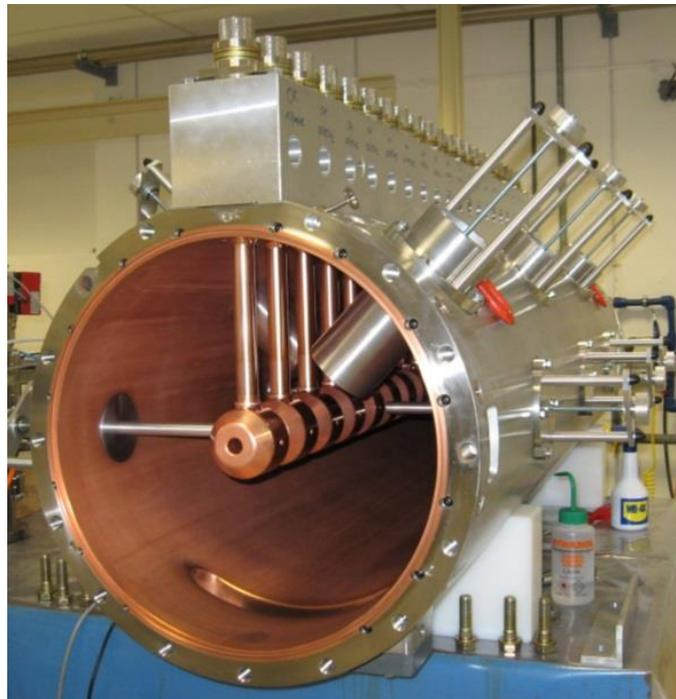
CERN LINAC 4: 352 MHz frequency, Tank diameter 500
