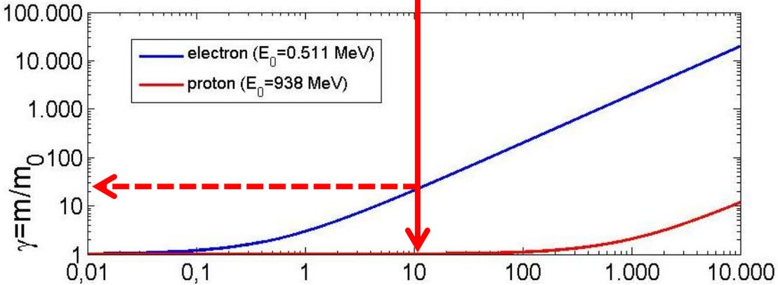
⇒ **Light particles (as electrons)** are practically fully relativistic ( $\beta \approx 1$ ,  $\gamma \gg 1$ ) at relatively low energy and **reach a constant velocity** ( $\sim c$ ). The acceleration process occurs at constant particle velocity
