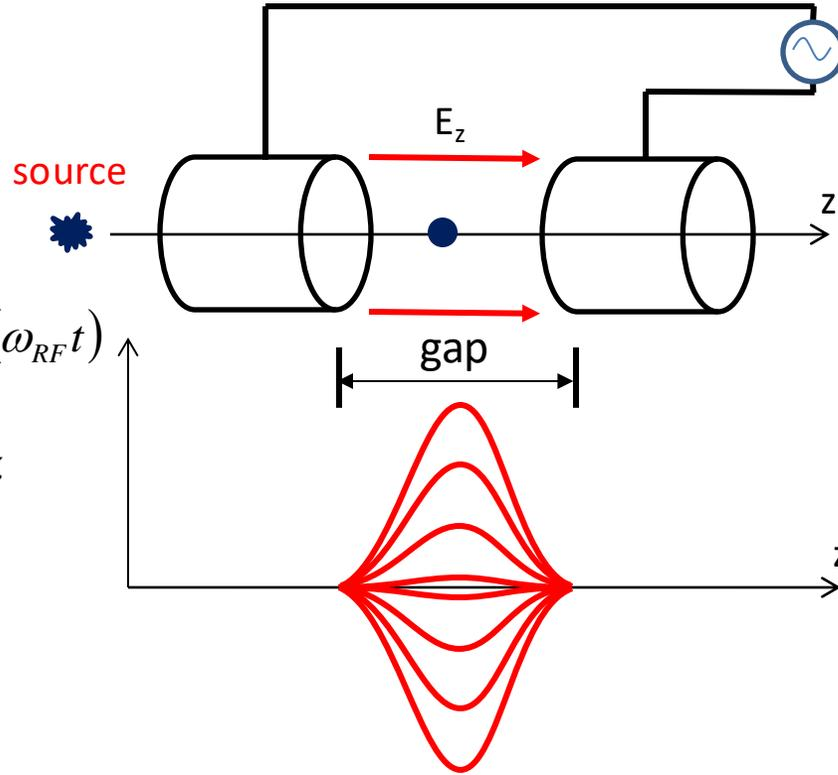
$$\Delta V = V_{RF} \cos(\omega_{RF} t) \quad \omega_{RF} = 2\pi f_{RF} = \frac{2\pi}{T_{RF}}$$
