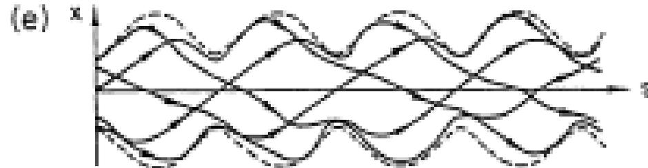
The area in the phase space occupied by the bunch is called **transverse emittance**
